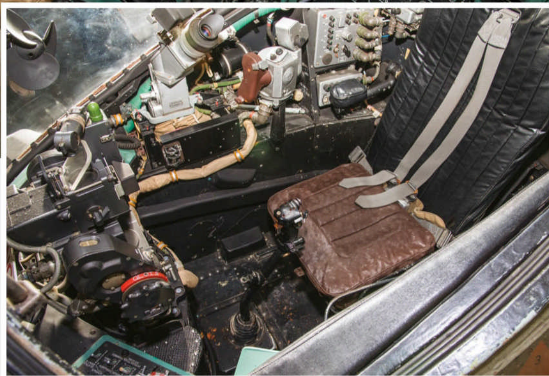
Right: The two occupants of the Mi-24, pilot and weapons operator, occupy tandem, stepped cockpits
